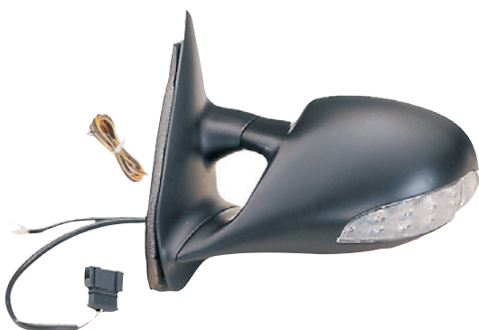
TH-805-04 R/L ELECTRIC, HEATED, W/LED LAMP
